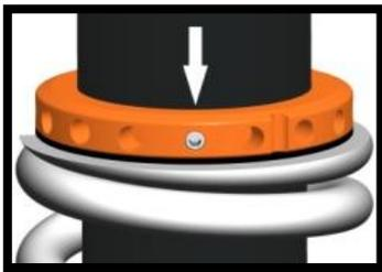
2) Mechanical Preload Adjuster with contra nut.
