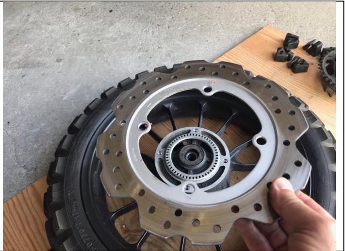
7. Remove the 4 shoulder bolts holding the OEM rear disc and ABS ring to the cast wheel, then transfer these to the new spoked wheel, note that the ABS ring goes on first next to the hub face, with the rear brake disc on top. Apply Loctite to the thread of the shoulder screws before inserting, torque to 40Nm.
