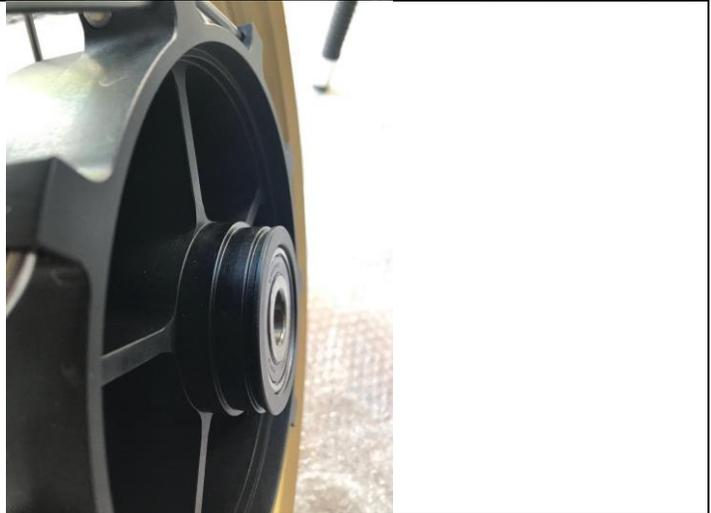
9. Push the sprocket and cush drive assembly into the new spoked wheel and insert the OEM spacer into the disc side of the wheel before inserting the new wheel back into the swinging arm.
