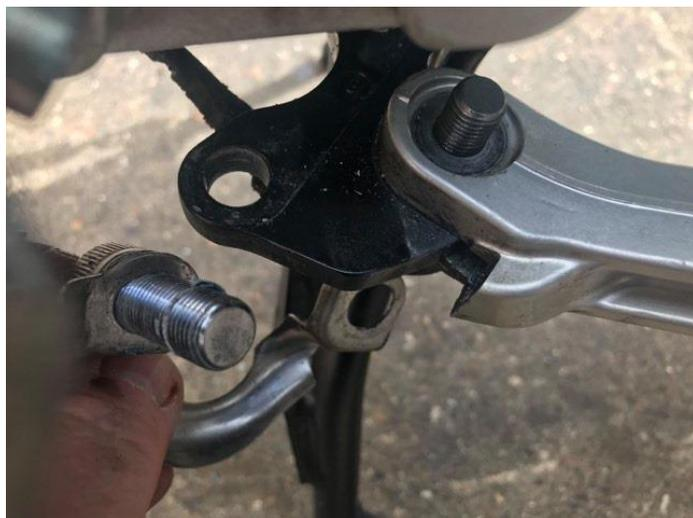
5. Turn over stand and bracket, then remove M6 switch bolt, using 10mm spanner.
