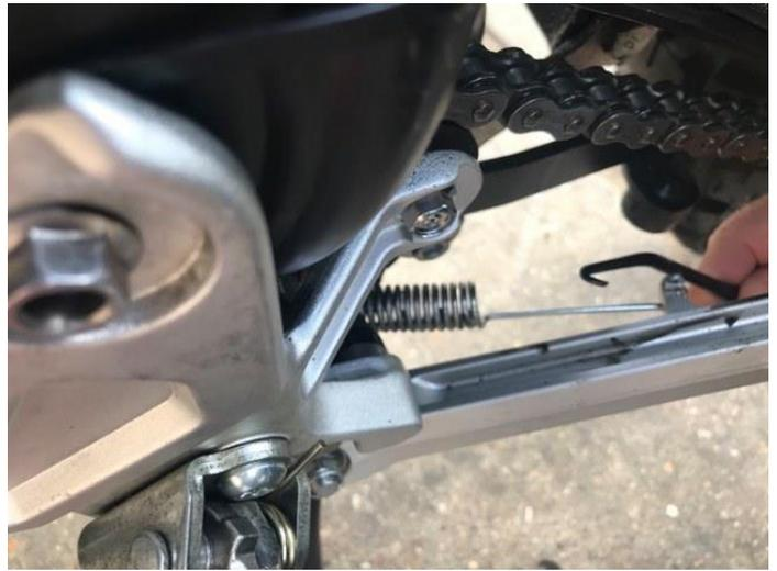
2. Using 14mm spanner, undo and remove nut on stand pivot bolt, as shown.
