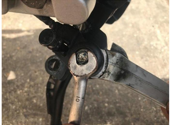
6. Remove switch and note position of small metal tab on underside of switch.
