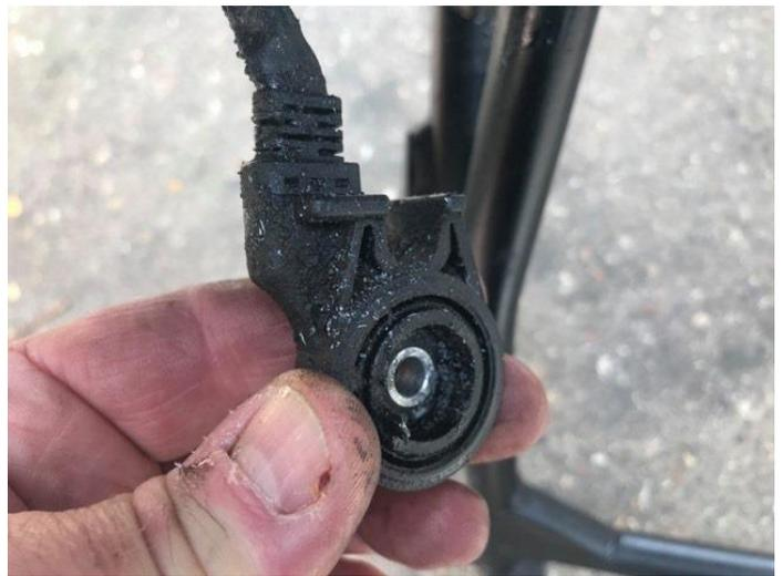
7. Remove pivot bolt using 13mm spanner, then discard OEM side stand, and clean pivot bracket before re-assembly.
