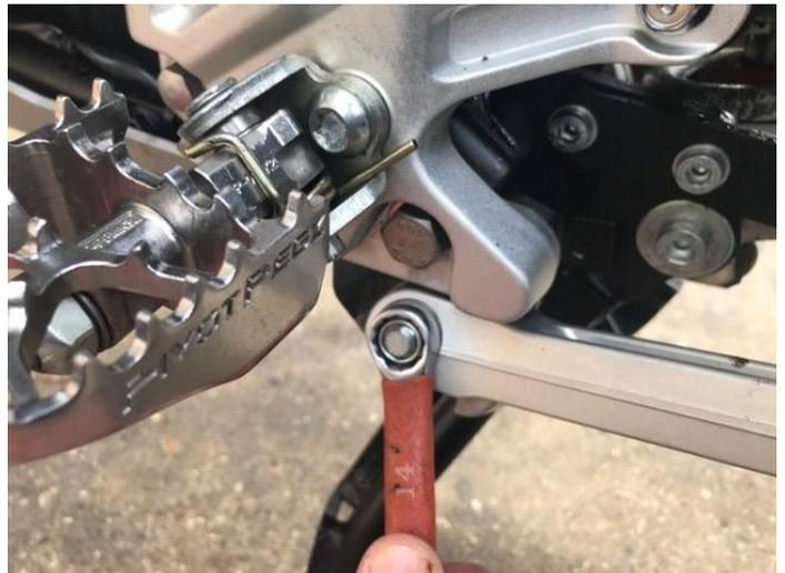
3. Using 10mm hex Allen key (if no centre stand fitted) or 10mm hex bit and 10mm ratchet ring spanner (if centre stand fitted) to undo and remove rear pivot bracket bolt.
