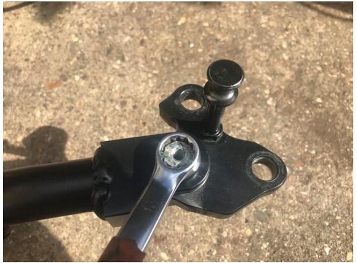
9. Offer switch onto head of pivot bolt and be very careful to ensure metal tab on switch aligns with slot in stand, as shown, and the slot on switch fits around peg on bracket.
