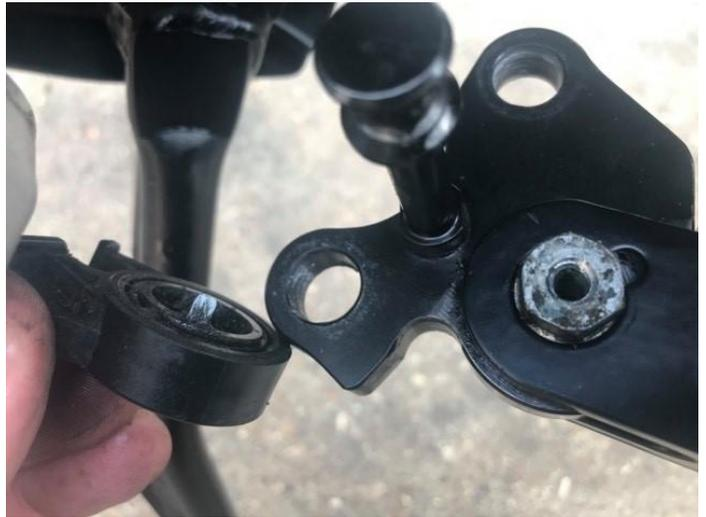
10. Apply Loctite to M6 switch bolt and tighten switch to stand assembly, check for free movement of new stand on bracket.
