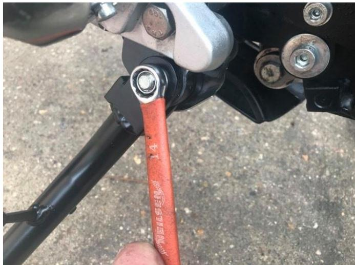
13. Attach new spring onto peg of pivot bracket, using shortest end of spring. Then, using tool provided, and with stand in "up" position, stretch spring to attach onto stand, as shown.
