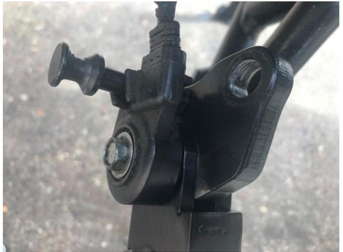
11. Apply Loctite to both M10 hanger bolts, then refit stand assembly onto footrest hanger, using front bolt first, with metal cover plate, tighten gently, then attach rear of bracket with second bolt, then fully tighten both bolts.
