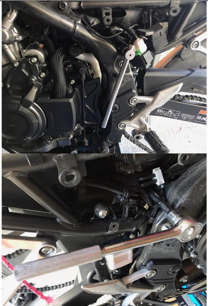
6. Using a long drift, or screwdriver, push out M10x48mm top bolt, whilst supporting shock body. Gently lower shock out of frame.
