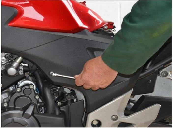
3. Undo both of the 17mm nuts on the flat steel dog bones, and then remove both M10 bolts, one attaching the dog bones to the underside of the swinging arm and the other end attaching to the OEM billet linkage. Retain both steel dog bones.
