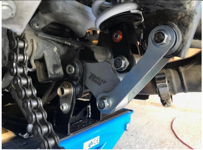
11. Attach lower shock mount to the new link (with new shorter bush fitted). Using the OEM M10 bolt and nut, but with the short spacers provided, one either side of the lower shock mount. Tighten to 40nm.
