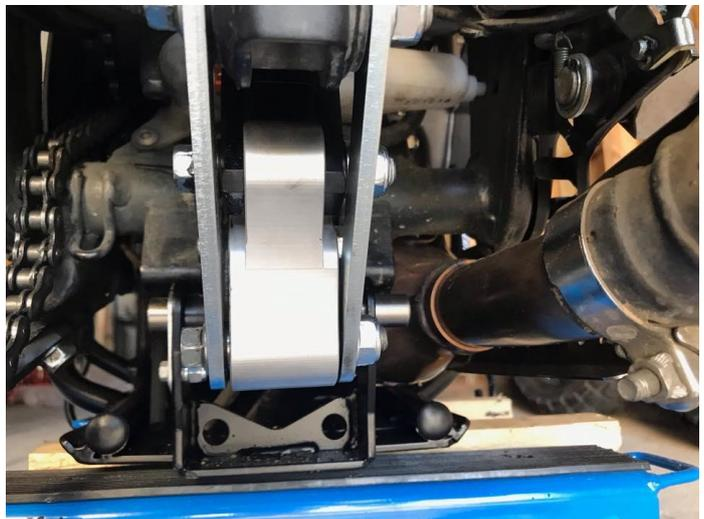
4. Undo 17mm nut on shock lower mount and remove M10 bolt. Allow OEM billet suspension link to drop down and undo 17mm nut from M10x58mm bolt securing link to frame, use 8mm Allen key to hold head of bolt. Remove bolt and remove two steel bushes from the OEM link to re-use in new link, discard the third bush. Insert both OEM steel bushes into new link, with grease and insert the new shorter bush into the new billet link where the suspension attaches, at its narrowest point.
