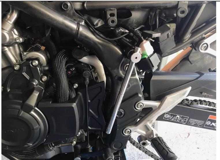
10. Fit new lower link and insert front M10x58mm bolt, tighten M10 nut (no washer) to 40Nm, using 8mm Allen key and 17mm socket.
