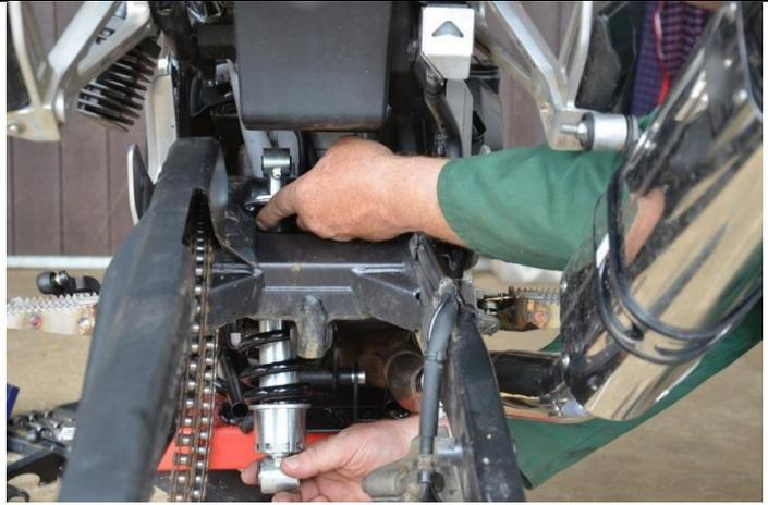
7. Insert new shock up through gap between swinging arm brace and rear of engine,
